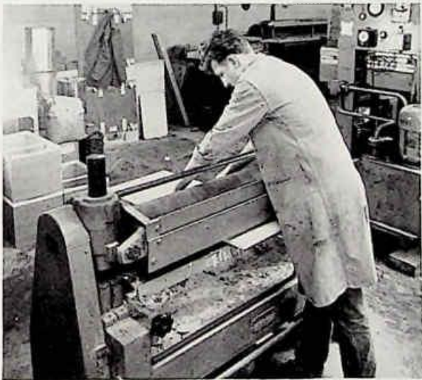
FIG. 4/3. Machine for spreading cold glue by rollers.
