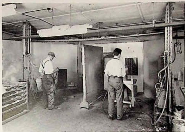
FIG. 7/3. Polyester spraying with ducts to supply exact mixture of accelerator and finishing material.
