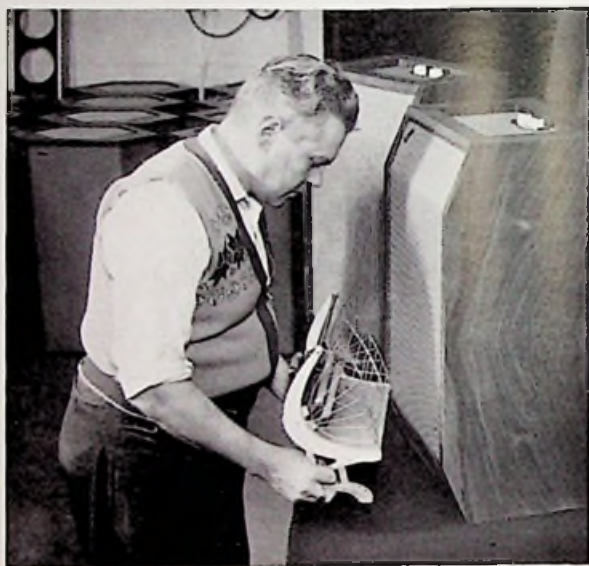
FIG. 8/3. Removing electric radiator after heat treatment of Tygan. At least 12 hours should be allowed for adhesive to set before this shrinkage is applied.
