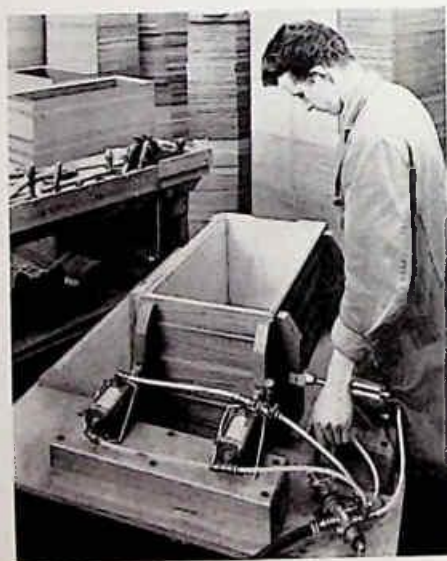
FIG. 5/7. Hydraulic assembly jig used with cold PVA adhesive. Setting time ten minutes.
